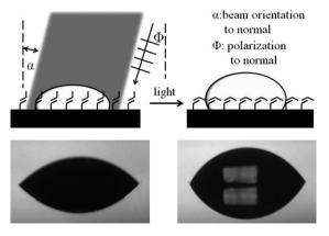
**Fig. 2** A schematic depiction of the photo-reversible surface effect and corresponding photo measurements of contact angles.
