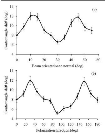
Fig. 3 Dependence of the two irradiation parameters influencing the water contact angle shift: (a) incoming beam direction (polarization direction was fixed to  $0^{\circ}$ ) and (b) polarization axis (incoming beam direction was fixed to normal). Irradiation was 70 mW cm<sup>-2</sup> at 488 nm for 30 s. The film thickness was 100 nm, and the initial contact angle was  $62^{\circ}$ .
