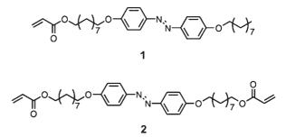
**Scheme 1.** Chemical structures of the LC monomer (1) and LC diacrylate (2) used in this study. Upon cooling, 1 changes from an isotropic to a smectic phase at 92 °C, and at 60 °C it becomes crystalline; upon cooling, 2 changes from an isotropic to a smectic phase at 91 °C, and at 74 °C it becomes crystalline; upon cooling, the mixture of 1/2 (20/80 mol/mol) changes from an isotropic to a smectic phase 89 °C, and at 60 °C it becomes crystalline.
