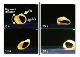
**Figure 1.** Photoinduced rolling motion of a continuous ring of LCE film. Series of photographs showing time profiles of the photoinduced rolling motion of the LCE ring by simultaneous irradiation with UV (366 nm, 200 mWcm<sup>-2</sup>) and visible light (>500 nm, 120 mWcm<sup>-2</sup>) at room temperature. Size of the LCE ring: 18 mm×3 mm (diameter: 6 mm). Thickness of the LCE ring: 20  $\mu$ m.
