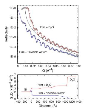
FIG. 6. (Color online). Neutron reflectivity data (top) of thin films composed of weak polyelectrolytes fabricated electrostatically onto a Si substrate in  $D_2O$  and invisible, or commonly referred-to, "contrast matched" water (92:8  $H_2O:D_2O$ ). One-dimensional SLD profiles (bottom) of poly-(acrylic acid) and poly(allyl)amine hydrochloride in pure  $D_2O$  and 92:8  $H_2O:D_2O$ .
