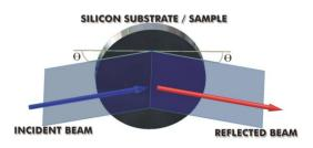
FIG. 1. (Color online). Reflection geometry showing the incident monochromatic neutron beam impinging on a silicon substrate at an angle  $\Theta$  and subsequently reflected at an equal angle  $\Theta$ . The angle between the straight through beam and the reflected beam is  $2\Theta$ .
