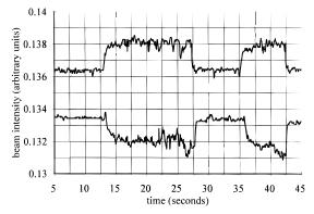
**Figure 5.** Change in beam intensity to demonstrate asymmetric two beam coupling in a PAC-5 photorefractive grating: top, intensity of beam 1; bottom, intensity of beam 2, as the other beam in introduced and removed.
