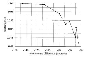
**Figure 3.** Maximum level of birefringence photoinducible vs  $T - T_{g}$ .
