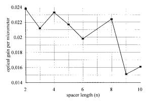
**Figure 6.** Optical gain acheivable for the PAC-*n* photorefractive polymers.
