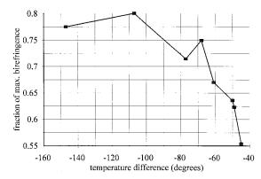
**Figure 4.** Fraction of photoinduced birefringence remaining after relaxation vs  $T - T_{g}$ .
