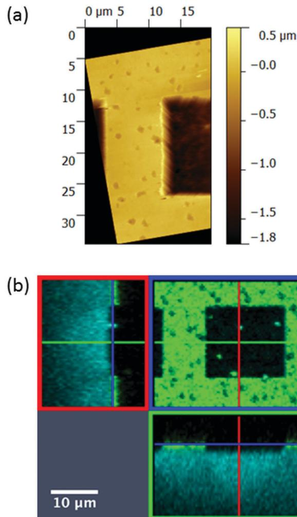
Fig. 2 (a) AFM image of photo-inscribed areas of azosilk (b) the corresponding confocal image. Blue channel: fluorescence at 488 nm excitation. Green channel: reflectance image. The blister top has completely separated from surface in this case.
