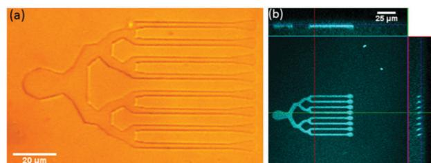
Fig. 3 (a) Wide field image of a microfluidic-inspired pattern made through the ocular of the microscope, demonstrating that the photo-inscribed structures can be easily visualized with an ordinary wide field microscope, so they can be readily found for later processing. (b) Cross sectional image of a microfluidic pattern written within the hydrated azosilk film showing the increased fluorescence obtained by irradiating several regions of interest.
