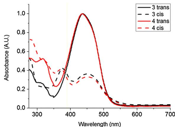
**Fig. 2.** Normalized UV–vis traces of Compounds **3** and **4** in the *trans* and *cis* photostationary states, demonstrating near-identical absorbances at the  $\pi\text{--}\pi^*$  azo transitions in the visible region >400 nm, but different absorbances in the UV due to the presence of the nitrobenzene moiety clicked on.
