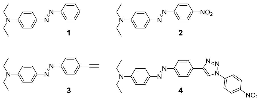
**Scheme 1.** Structures used to validate the ‘click’ approach to diversify azobenzenes. A model diethylaniline dye (**1**), a diethylaniline disperse red 1 dye (**2**), the ‘clickable’ diethylaniline derivative (**3**), and a ‘clicked’ nitrobenzene product (**4**).
