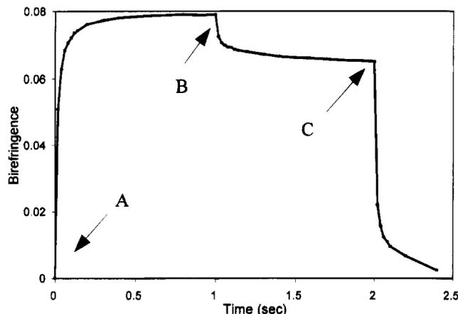
**Figure 1.** Typical write/erase curve on a polyDR1A film. The structure of the polymer is shown in Chart 1. At point A, a plane polarized laser (514 nm) is turned on; at point B it is turned off; at point C the same laser, but circularly polarized, is turned on for erasure.
