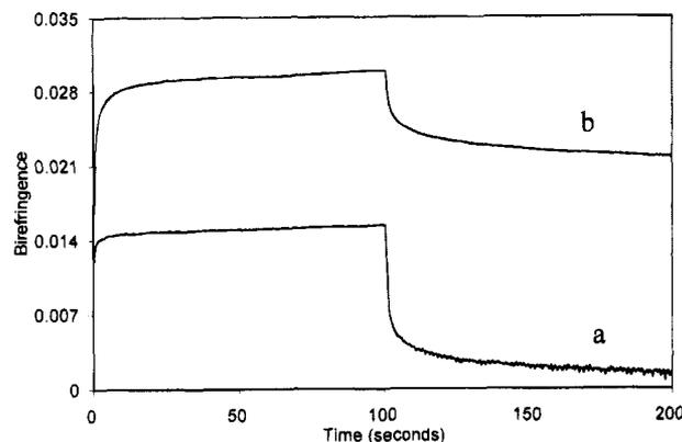
**Figure 2.** Photoinduced birefringence on (a) a film of 12 mol % DR1 in pMMA of 1313 nm thickness and (b) a film of 41 mol % DR1 in pASH of 530 nm thickness. The writing laser is turned on at time zero and off at 100 s.
