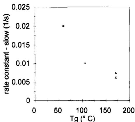
**Figure 4.** Rate constant of the birefringence decay after 110 s after the laser has been switched off as a function of the  $T_g$  of the sample: (■) DR1 in pMMA; (□) p(DR1A-co-MMA); (▲) DR1 in pASH, and (×) pDR1A-*b*-pMMA.
