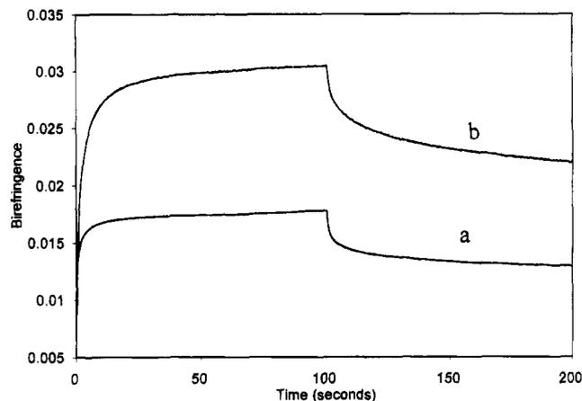
**Figure 3.** Photoinduced birefringence on (a) a film of a blend of pASH with pDR1A containing 39 mol % pDRA1 of 1783 nm thickness and (b) a film of poly(DR1A-co-MMA) copolymer containing 8 mol % DR1A of 2783 nm thickness. The writing laser is turned on at time zero and off at 100 s.
