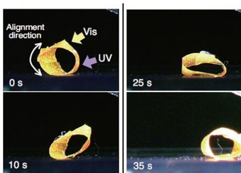
**Figure 1.** Photoinduced rolling motion of a continuous ring of LCE film. Series of photographs showing time profiles of the photoinduced rolling motion of the LCE ring by simultaneous irradiation with UV (366 nm,  $200 \text{ mWcm}^{-2}$ ) and visible light ( $> 500 \text{ nm}$ ,  $120 \text{ mWcm}^{-2}$ ) at room temperature. Size of the LCE ring:  $18 \text{ mm} \times 3 \text{ mm}$  (diameter:  $6 \text{ mm}$ ). Thickness of the LCE ring:  $20 \mu\text{m}$ .
