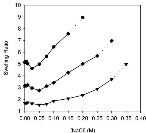
**Figure 8.** Effect of the NaCl concentration in the swelling medium (pH 7.0) on the ratio of film swelling for films assembled at pH 4.0 (●), pH 7.0 (▼), and pH 10.0 (◆). The dotted line indicates the onset of film decomposition. The uncertainty in the swelling ratio is  $\pm 0.4$ –1.2%.
