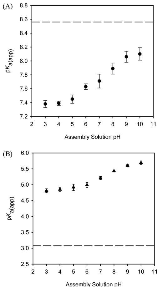
**Figure 4.** Dependence of the  $pK_{a(\text{app})}$  of (A) (PAH/HA)<sub>5.5</sub> and (B) (PAH/HA)<sub>6</sub> on the assembly solution pH. The dashed lines indicate the dilute solution  $pK_{a(\text{app})}$ .
