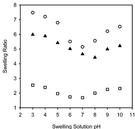
**Figure 7.** Influence of the swelling solution pH on the degree of (PAH/HA)<sub>15</sub> film swelling for films assembled at pH 4.0 (○), pH 7.0 (□), and pH 10.0 (▲). The uncertainty in the swelling ratio is  $\pm 0.6$ –1.0%.
