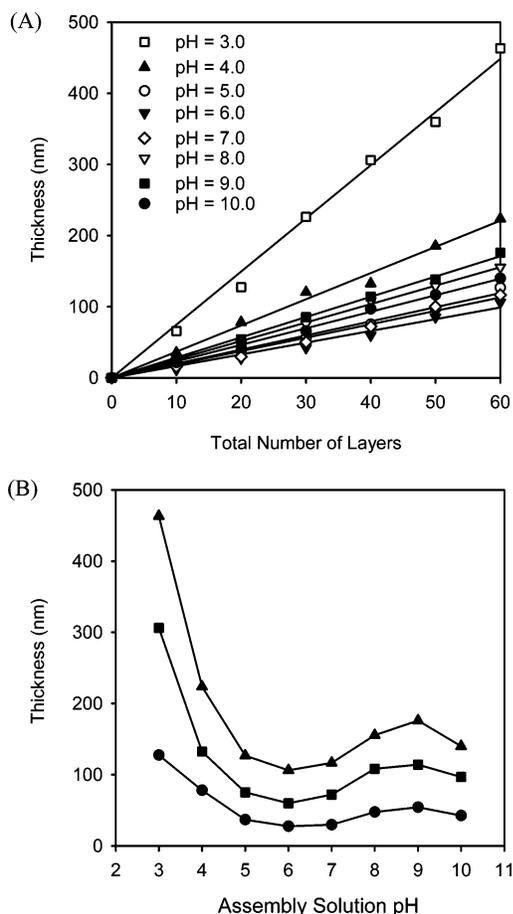
**Figure 2.** (A) Profile of the dry thickness of PAH/HA films assembled at different pH values as a function of the total number of layers in the film. (B) Dry film thickness of (PAH/HA)<sub>10</sub> (●), (PAH/HA)<sub>20</sub> (■), and (PAH/HA)<sub>30</sub> (▲) films versus assembly solution pH. The uncertainty in the thickness is  $\pm 1.2$ – $2.5\%$ , and for the swelling ratio it is  $\pm 0.8$ – $1.4\%$ .
