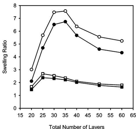
**Figure 5.** Influence of the film thickness on the swelling ratio for a film assembled at pH 4.0 (circles) and pH 7.0 (squares): swelling solution pH 3.0 (open symbols) and pH 9.0 (closed symbols). The dry film thickness is indicated numerically for films with a given total number of layers. The uncertainty in the thickness is  $\pm 1.2$ – $1.8\%$ , and that for the swelling ratio is  $\pm 0.4$ – $1.5\%$ .
