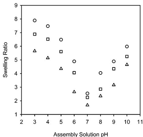
**Figure 6.** Dependence of the swelling ratio on the assembly pH conditions for films exposed to solutions of pH 3.0 (○), pH 7.0 (△), and pH 9.0 (□). The uncertainty in the swelling ratio is  $\pm 0.7$ – $1.1\%$ .
