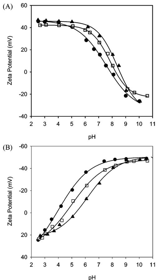
**Figure 3.** Some example titration curves for (A) (PAH/HA)<sub>5.5</sub> and (B) (PAH/HA)<sub>6</sub> assembled at pH 4.0 (●), pH 7.0 (□), and pH 10.0 (▲). The uncertainty in  $pK_{a(\text{app})}$  is  $\pm 0.03$ – $0.09$ .
