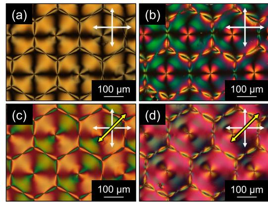
**Fig. 3.** Polarized optical micrographs of a film with (a), (c)  $R = 196\ \text{nm}$ , and (b), (d)  $R = 400\ \text{nm}$ . Polarized optical micrographs of resultant polymer films under crossed polarizers either without (a), (b), or with (c), (d) a test plate with a retardation of  $530\ \text{nm}$ . White arrows show the direction of polarizers. Yellow arrows indicate the optical axis of the test plate.
