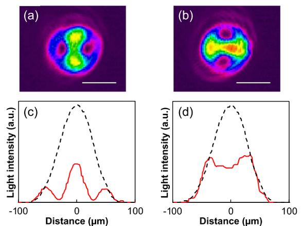
**Fig. 4.** (a), (b) Measured beam shape through a film with  $R = 196\ \text{nm}$  and  $R = 400\ \text{nm}$ , respectively. Scale bar =  $100\ \mu\text{m}$ . (c), (d) One-dimensional intensity profiles of the incident laser beam (black broken line), and transmitted light through a film with  $R = 196\ \text{nm}$  and  $R = 400\ \text{nm}$ , respectively (red line).
