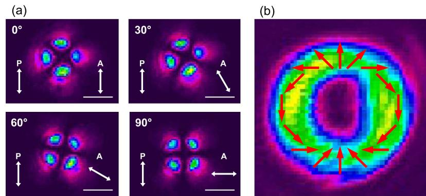
**Fig. 5.** (a) Beam profile of a film with  $R = 326$  nm observed through an analyzer. (b) Optical axis distribution of the doughnut beam detected. Scale bar = 100  $\mu\text{m}$ .
