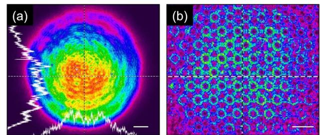
**Fig. 6.** (a) Beam profile of the incident light and (b) transmitted light through the polymer film with array patterns. Scale bar = 500  $\mu\text{m}$ .
